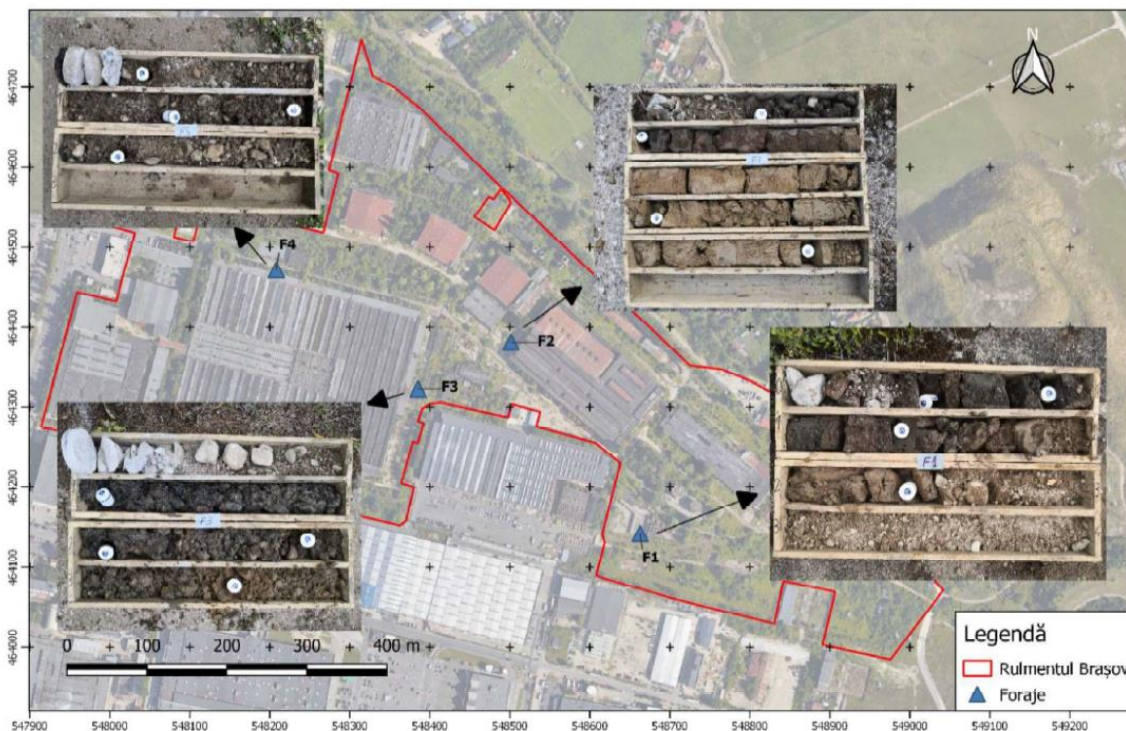
Figure 25 - Location of boreholes drilled and rocks extracted by depth intervals
